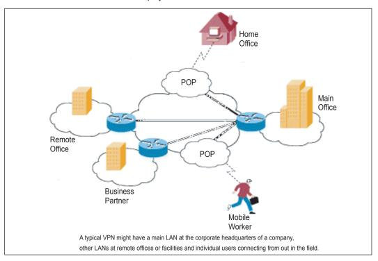
Basically, a VPN is a private network that uses a public network (usually the Internet) to connect remote sites or users together. Instead of using a dedicated, real-world connection such as leased line, a VPN uses "virtual" connections routed through the Internet from the company's private network to the remote site or employee. In this edition, you will gain a fundamental understanding of VPNs, and learn about basic VPN components, technologies, tunneling and security.
